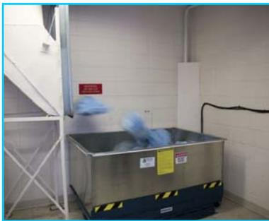
➡ This tilter unit was suggested by a safety-ergonomic team to reduce bending over the edge and reaching down into a wooden container to retrieve laundry bags. Now the stainless steel container is tilted up to allow easier removal of the bags. The unit was made to fit the room and height of the chute for improved ergonomics.
