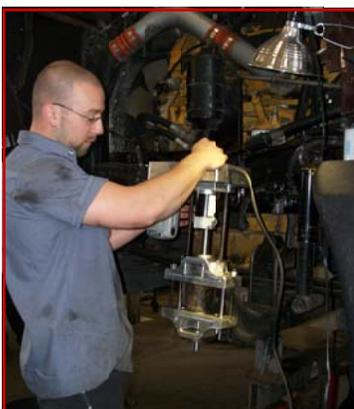
Chris Huntley, the Alignment Service Manager, and Brad Wood, an Alignment Technician, traveled to Ohio in April for training on the Axle Doctor: Steering Axle Boring and Sleeving System. We purchased the equipment and are able to perform this service in our shop or at the customer's location. This process can **save the customer time and money** by repairing the axle eye instead of replacing the axle! For more information or to set up an appointment call Chris at: (616) 669-8700.
